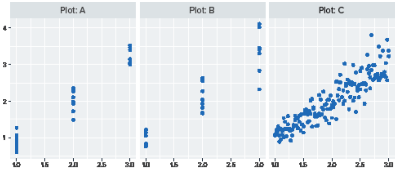
Figure 2 – Plot A illustrates constant variance. Plots B and C illustrate non-constant variance.
